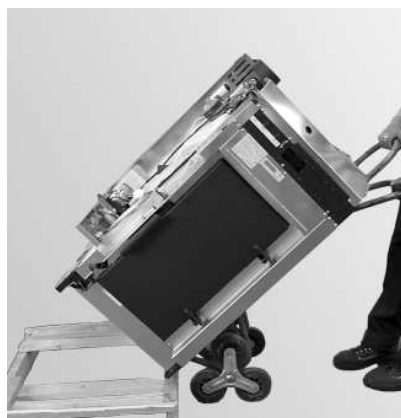
Fig. 12 Lift boiler off pallet with sack truck
