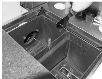
Fig. 57 Clean the heat exchangers
