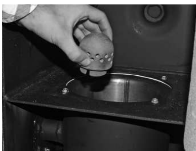
Fig. 45 Take out the primary air pin
