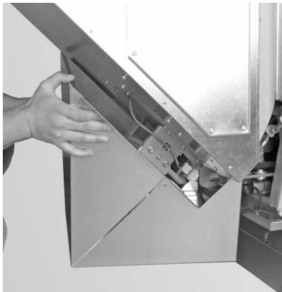
Fig. 54 Hook cover into place
