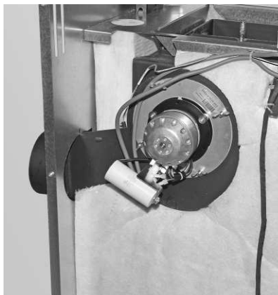
Fig. 33 Re-screw the induced draught fan into place adjusted by 90°
