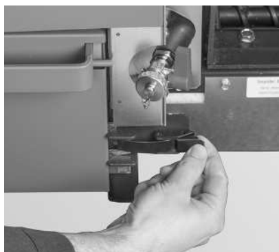
Fig. 101 Close the ash box fastener
