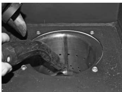
Fig. 44 Vacuum out the burner bowl
